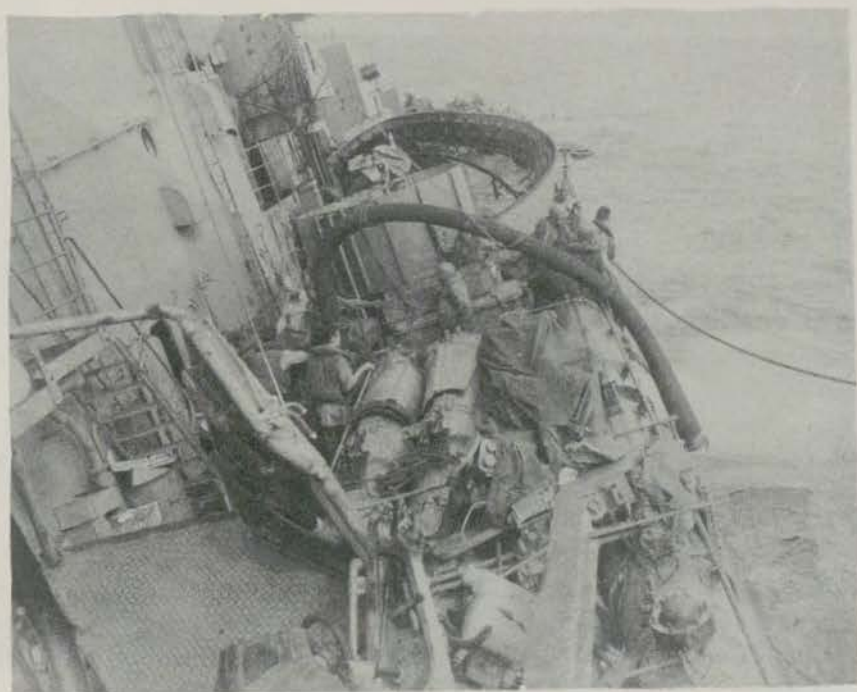
Photo 2: Looking aft on port side showing damaged 40mm and torpedo tube mounts. Discharge line from 6-inch pump in B-207-L visible. Ship has starboard list.
