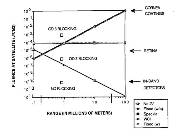
EFFECT OF BAND-BLOCKING FILTERS ON SENSOR FLUENCE DAMAGE THRESHOLDS
